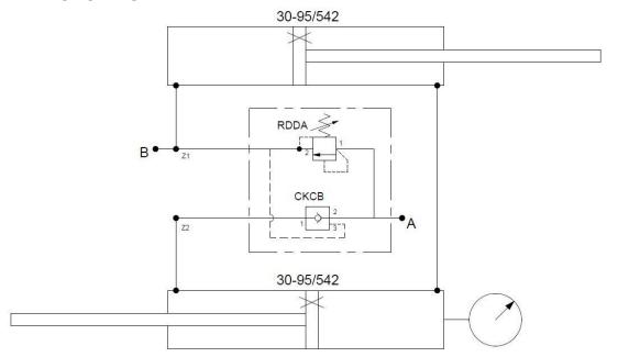
33000003- hydraulic block; RDDA-relief valve, CKCB- check valve.
